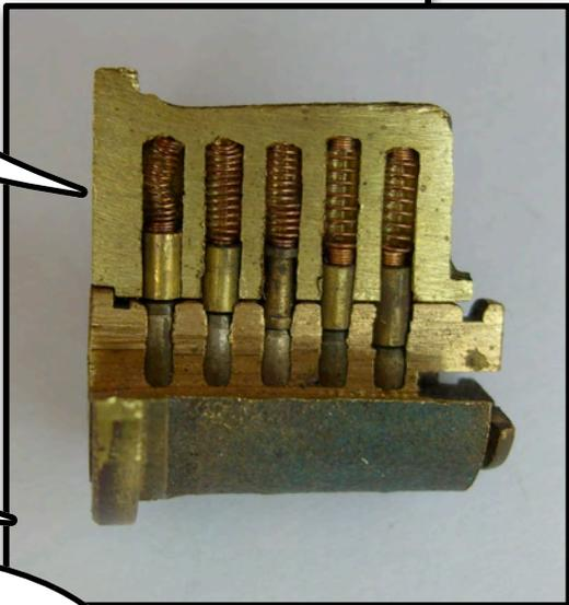
THE SHEAR LINE IS THE LINE WHERE THE TOP OF THE PLUG MEETS THE SHELL
