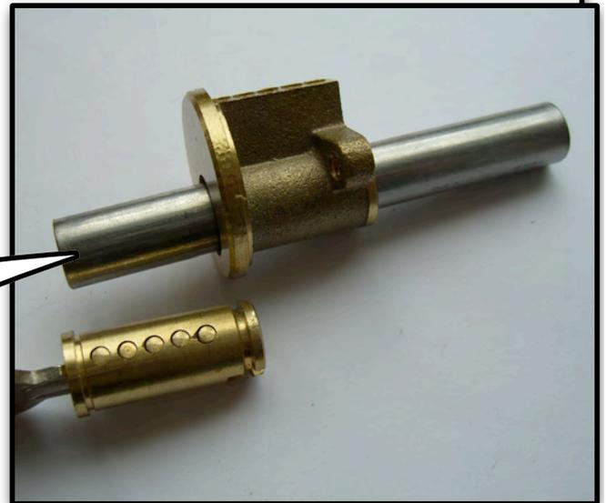
IN ORDER TO REMOVE THE PLUG, YOU WILL NEED A PLUG FOLLOWER. THESE CAN BE PURCHASED, OR MADE FROM WOODEN DOWEL. THERE ARE A VARIETY OF PLUG DIAMETERS, SO YOU WILL NEED A VARIETY OF PLUG FOLLOWERS. HOWEVER, THE MOST COMMON SIZE FOR LOCKS IN NORTH AMERICA IS 1/2 INCH.
