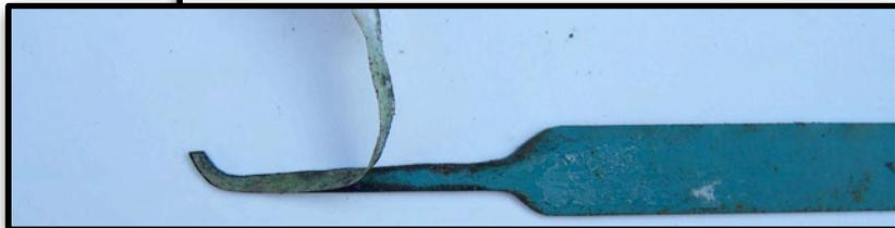
GRIND OUT THE BASIC SHAPE OF THE PICK. USE THE CORNERS OF THE GRIND WHEEL TO MAKE THE CURVED SHAPES. FOR FINER DETAIL, YOU MAY WISH TO USE A ROTARY TOOL (LIKE A DREMEL) WITH A CUTTING WHEEL TO GET THE SHAPE YOU WANT.
