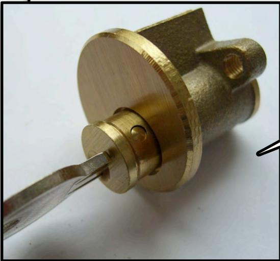
WITH THE KEY INSTALLED, AND THE CIRCLIP REMOVED, THE PLUG IS FREE TO BE REMOVED FROM THE SHELL
