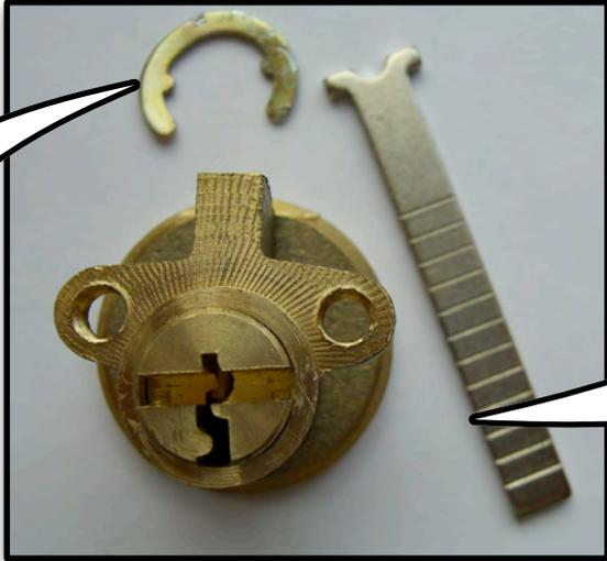
IN ORDER TO REMOVE THE PLUG, THE PIN STACKS MUST ALL BE LIFTED TO THE SHEAR LINE. THIS CAN BE DONE WITH THE CORRECT KEY, BY PICKING THE LOCK, OR WITH A THIN METAL SHIM
