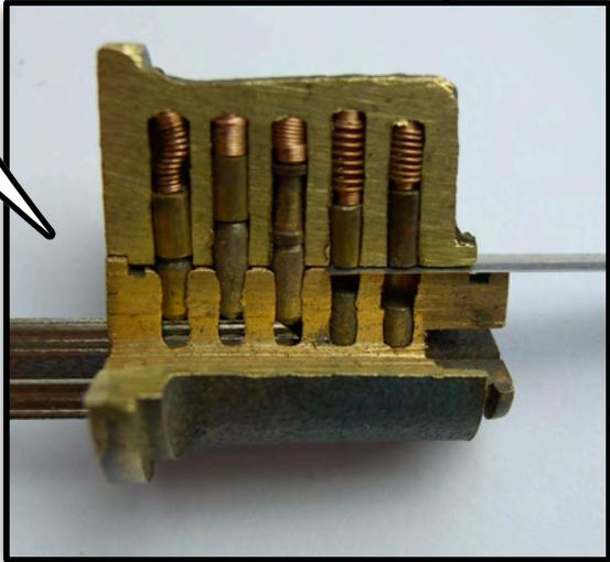
ONCE COMPLETED, YOUR SHIM WILL BE FULLY INSERTED INTO THE LOCK AND ALL THE DRIVER PINS WILL BE STUCK ABOVE THE SHEAR LINE. YOU ARE NOW ABLE TO REMOVE THE PLUG, BUT DON'T DO THAT YET! SEE THE NEXT PAGE FIRST!
